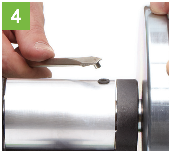
4 Using screwdriver, press magnet into grommet
