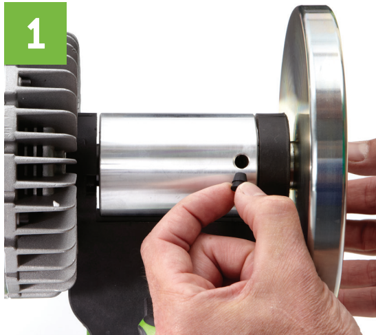
1 Insert rubber grommet into roller hole
