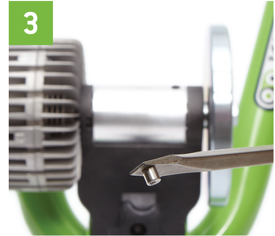
3 Snap magnet to standard screwdriver to firmly hold
