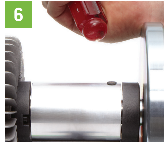
6 Magnet should be flush with top of grommet
