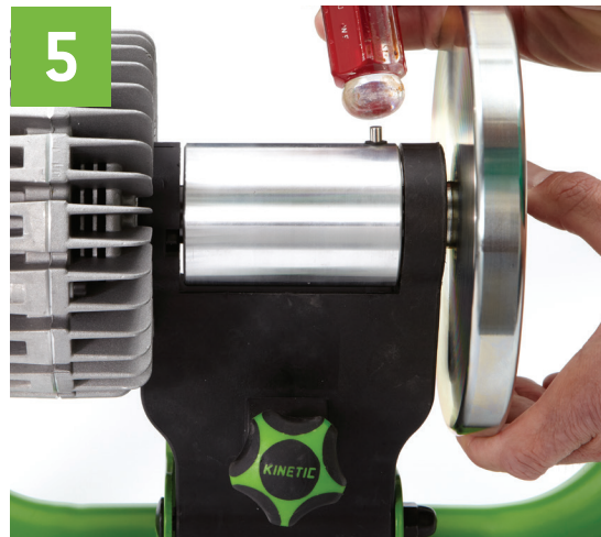
5 Press magnet flush with grommet using screwdriver
